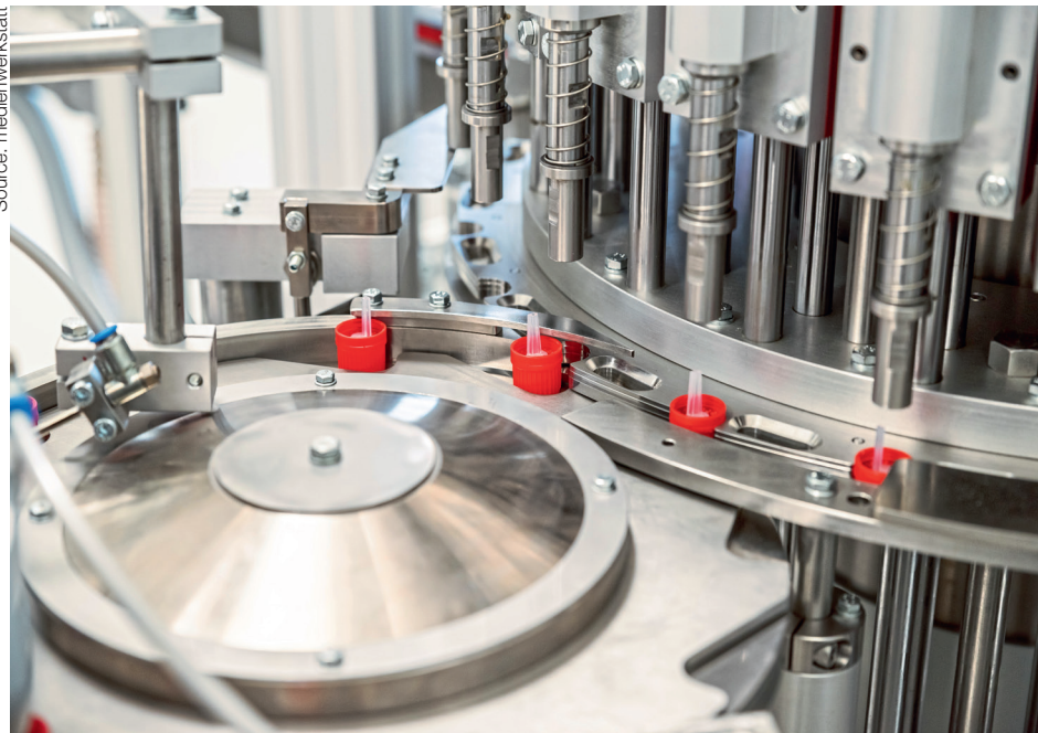
Once assembled, the dropper caps are subjected to a height check prior to sorting to remove non-compliant parts
